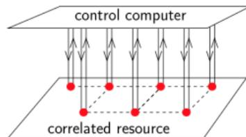
FIG. 1: The control computer provides one of  $k$  choices as the classical input (downward arrows) to each of the correlated parties (circles in the resource) and receives one of  $l$  choices as the output.
